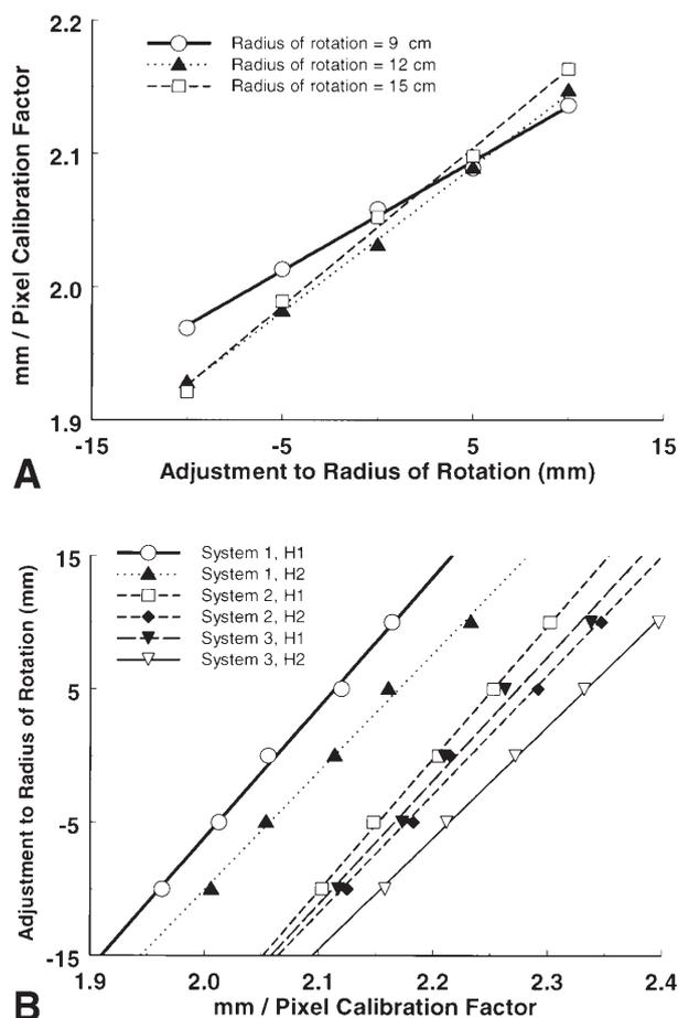
**Fig. 3.** **A** Effect of changes in the apparent system radius of rotation on image size (mm/pixel calibration factor) for studies acquired at three different radii of rotation on head 1 of system 1. **B** Adjustments to the radii of rotation required to obtain the same mm/pixel calibration factor on all six collimators
