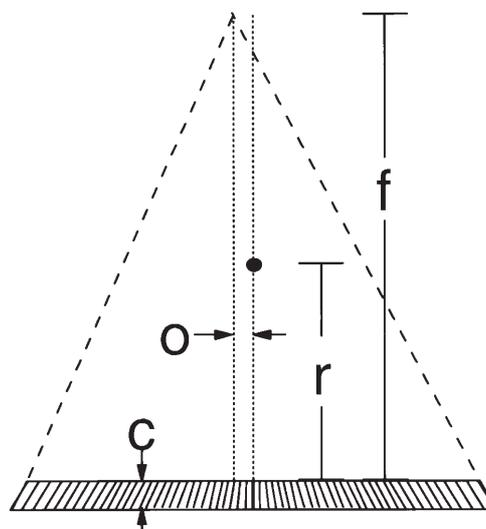
**Fig. 1.** Schematic diagram illustrating the various fan-beam collimator parameters that affect image size. These are:  $f$ , distance from focal line to collimator surface;  $c$ , collimator thickness;  $r$ , distance from center of rotation to collimator surface; and  $o$ , offset of focal line from center of rotation. For data reconstruction, collimator focal length =  $f+c$ , and radius of rotation =  $r+c$
