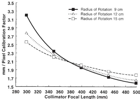
**Fig. 2.** Relationship between image size (mm/pixel calibration factor) and value for collimator focal length used in tomographic reconstruction, for studies acquired at three different radii of rotation. Results are shown for head 1, system 1 with a nominal collimator focal length of 407 mm
